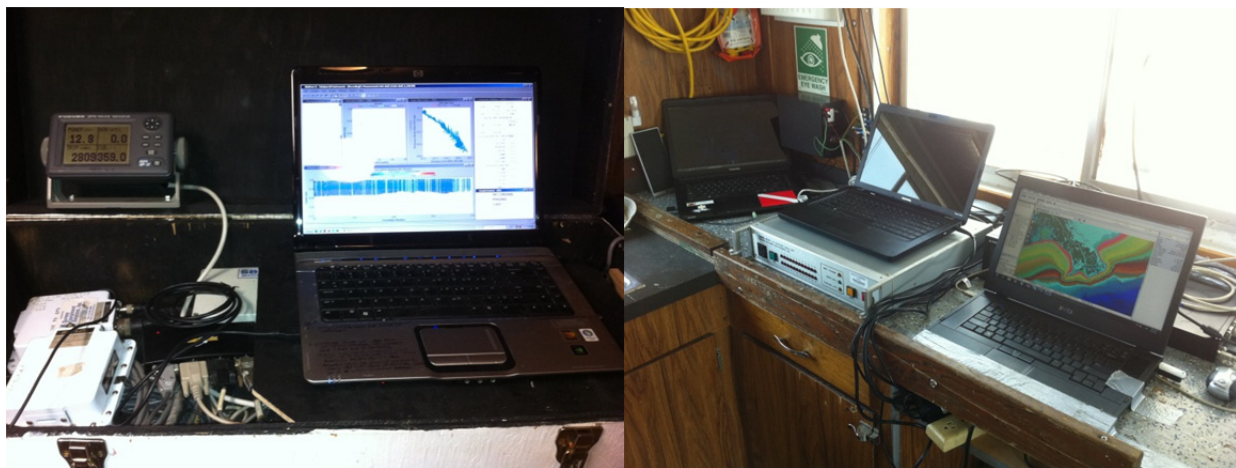
Figure 6. Real time ADCP acquisition station (left), Nav station (right).
