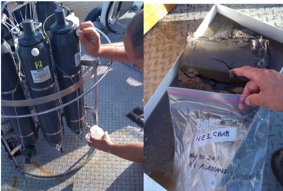
Figure 4. Water sampling (left), Ponar grab sampling (right).
